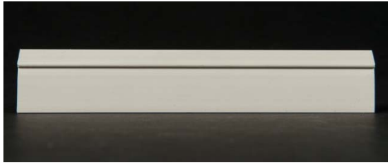
VaproTermination Bar is a rigid thermoplastic extrusion, non-corrosive, UV-resistant, rot-resistant, non-conductive, and 100% recycled. Material guide lip gives installers correct termination point. Available in 8' (2.4 M) L x 1" (25 mm) H x 1/8" (3 mm) D.
