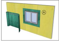
1. After flashing the window's rough opening, begin installation at the base of the wall, progressing in a shingle fashion upwards.
