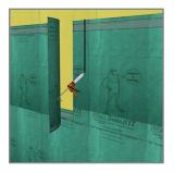
4. Overlap vertical seams by 12" minimum, seal with VaproLiqui-Flash or VaproBond Adhesive Sealant if necessary.
