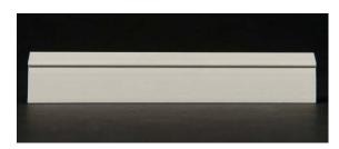
VaproTermination Bar is a rigid thermoplastic extrusion, non-corrosive, UV-resistant, rot-resistant, non-conductive, and 100% recycled. Material guide lip gives installers correct termination point. Available in 8' (2.4 M) L x 1" (25 mm) H x 1/8" (3 mm) D.
