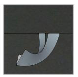
8. Line up both release films together so they can be pulled down the wall with one hand.
