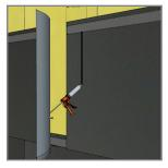
4. Overlap vertical seams by 12" minimum, seal with VaproBond Adhesive Sealant.
