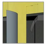
5. Remove release film from top of tape where flap overlaps.
